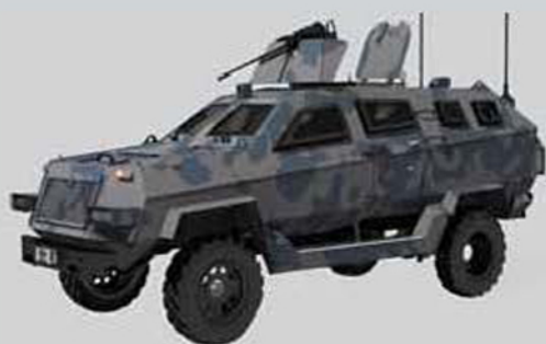
Open Turret with 12.7x108 mm NSV machinegun
