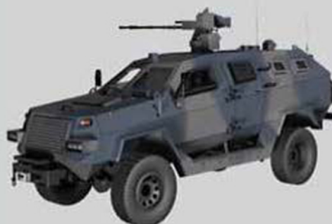
Fire support vehicle (14.5x114 mm KPVT)
